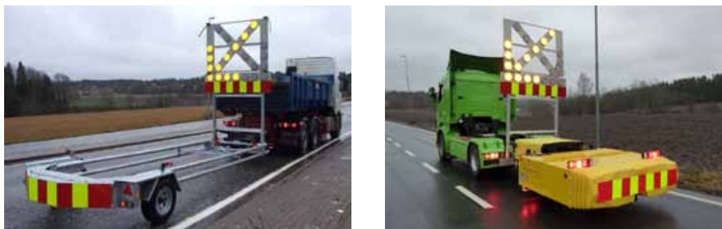
Figure 4.12 Energy absorbing equipment on vehicles (examples).
