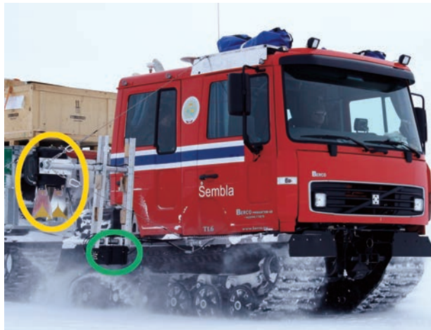
Fig. 1.1: C-band (green circle) and UWB radar (yellow circle) mounted on a TL-6 Berco tracked vehicle during the Norwegian-U.S. traverse across East Antarctica.
