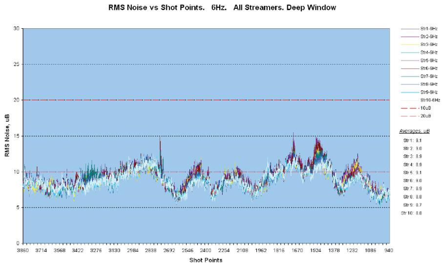
Figure 1.8: Top image: Shows the average rms-noise level on all 480 channels for 10 streamer cables. Bottom image: The average rms-level pr shot pr streamer during a line.
