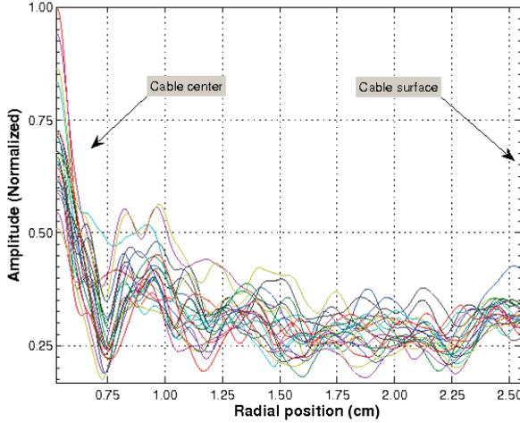
Figure 5.13: Flow noise levels as a function of distance from the center of a cable with diameter  $y^+ = 1440$ . On a real seismic streamer this roughly corresponds to a radius of 5.2 cm. The sharp increase towards the center is partly caused by a reflective boundary near the cylinder core used in the simulation.
