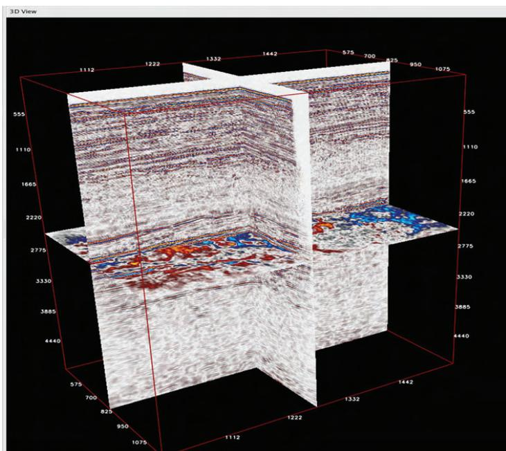
Figure 1.4: A seismic 3-D cube displayed through a number of 2-D planes. Time/depth increase downwards in this image, and the colors represent the magnitude of the reflection from geological features in the subsurface.
