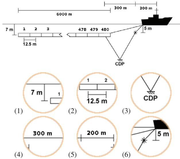
Figure 1.5: A simple but typical 2-D acquisition geometry adapted from a Fugro training program.
