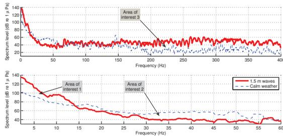
Figure 4.10: Power spectral estimates of noise records acquired on the streamer. The spectral estimates were obtained by using a multi-taper method. The bottom image is a zoom of the data in the range from 2 to 60 Hz. The steamer was at 5 m when the data were acquired, and the vessel velocity was 4.5 knots.
