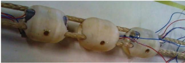
Figure 2.5: Parts of a hydrophone array during manufacturing.
