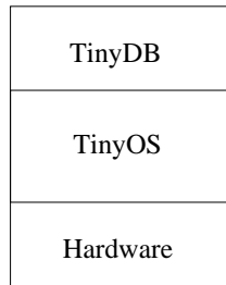
Figure 2.1: Schematic drawing of a TinyDB sensor mote.
