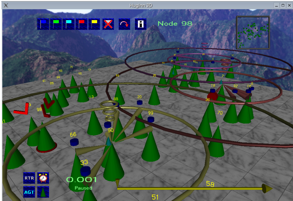
Figure 3.3: An image of Huginn showing nodes, transmission and carrier sensing ranges [51].
