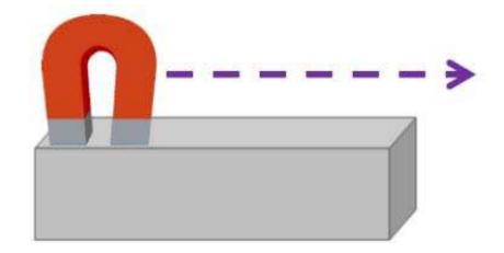
This introduces lines of magnetic flux into the specimen
