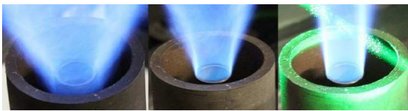
Figure 6: A photograph of the flame (angled view) as a function of swirl number. From left to right S=1.07 , 0.58 and 0.3.
