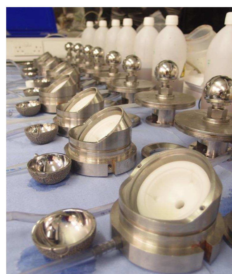
Figure 1. Ten Adept heads and cups with their holding fixtures.
