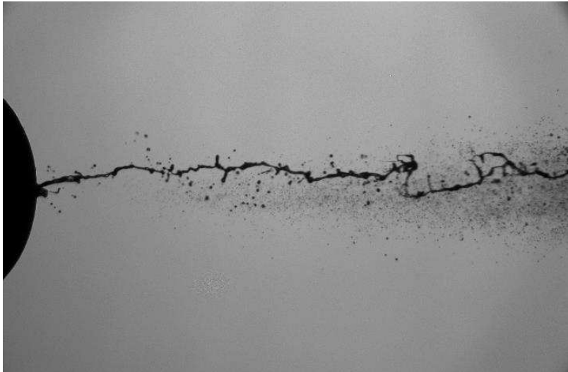
Ambient 1 bar, Injection 500 bar, n-dodecane
