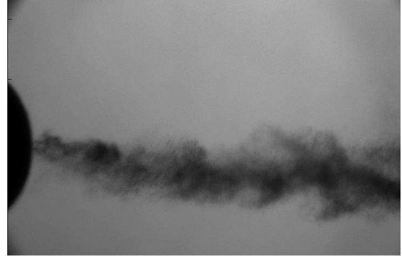
Ambient 40 bar, Injection 500 bar, n-dodecane
