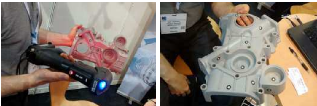
Figure 11: Creaform 300 demo showing high tolerance measurements
