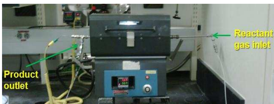
Figure 3.3. Stainless steel fixed bed and tube furnace.
