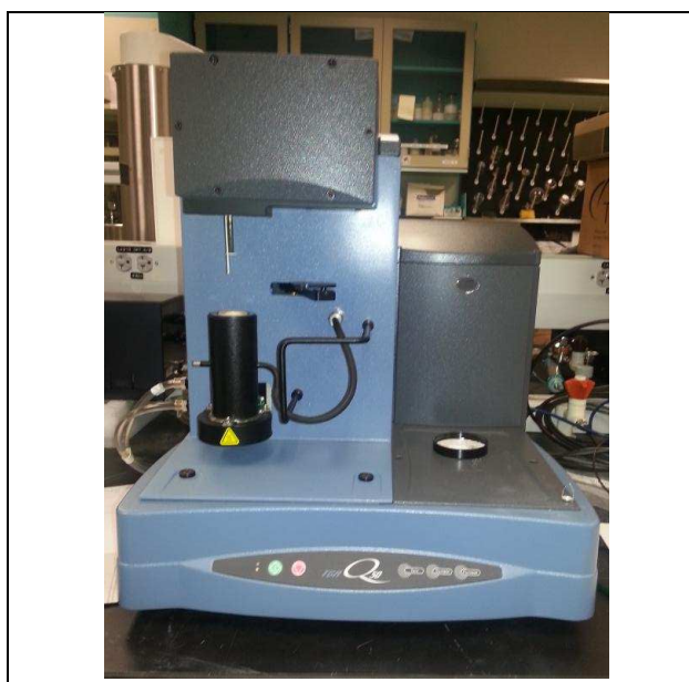
Figure 2.3. TGA instruments applied to study the carbonic deposition of selected catalyst
