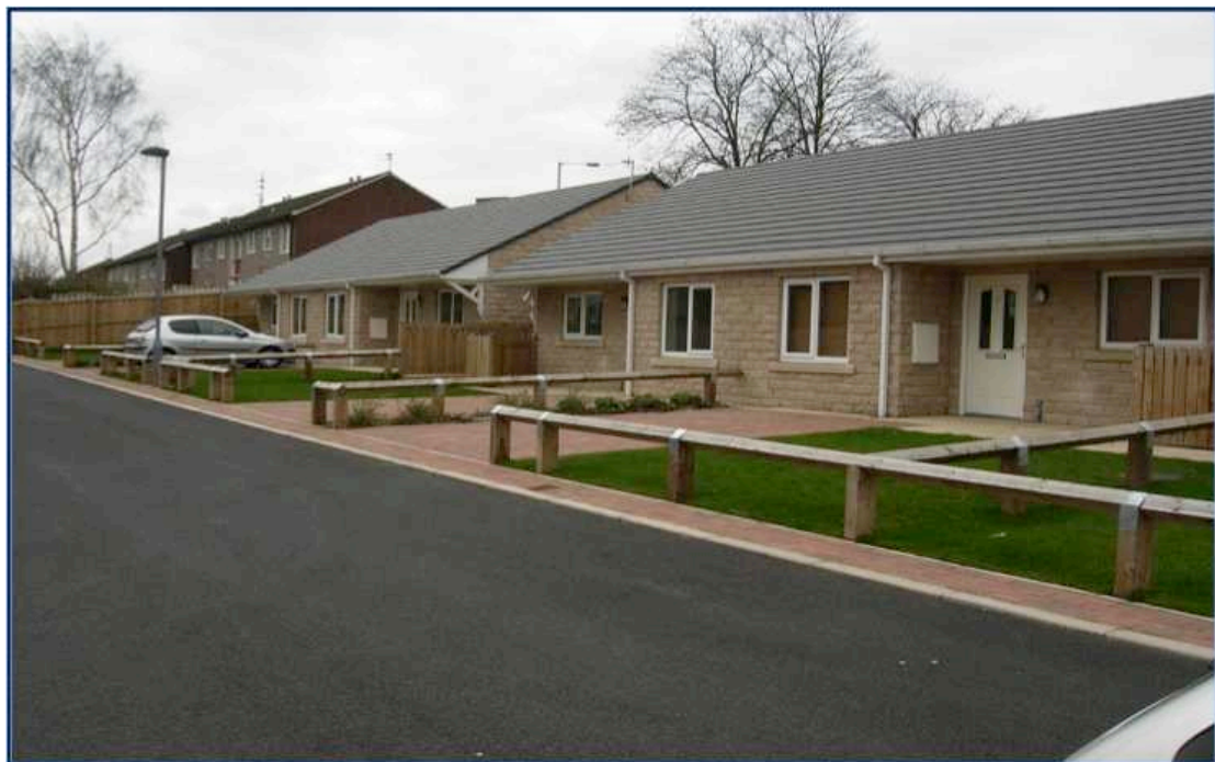
Figure 3: The semi-private space is clearly demarcated through a change in road colour and texture.
