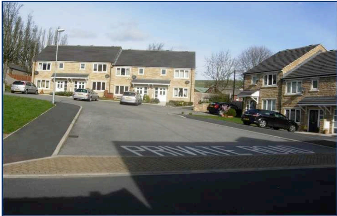
Figure 2: Creating a symbolic barrier through a change in road colour/texture
