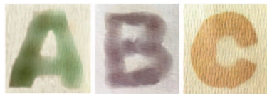
Fig. 5 Images of three sheets of white filter paper impregnated with optimal photochromic dye mixture and irradiated by UV-A (A), UV-B (B) (emitted by a 125 W Xe lamp) and UV-C (C) (emitted by a Hg lamp) radiation through negative masks reproducing the letters (A, B and C), respectively.
