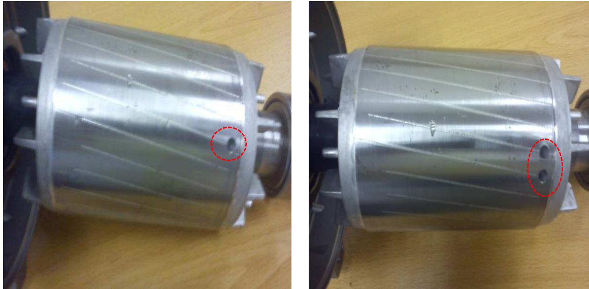
(a) Rotor with One Bar Broken
