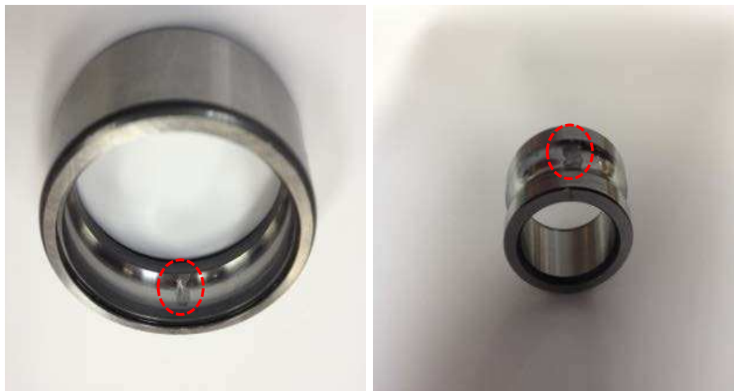
(a) Outer race fault
