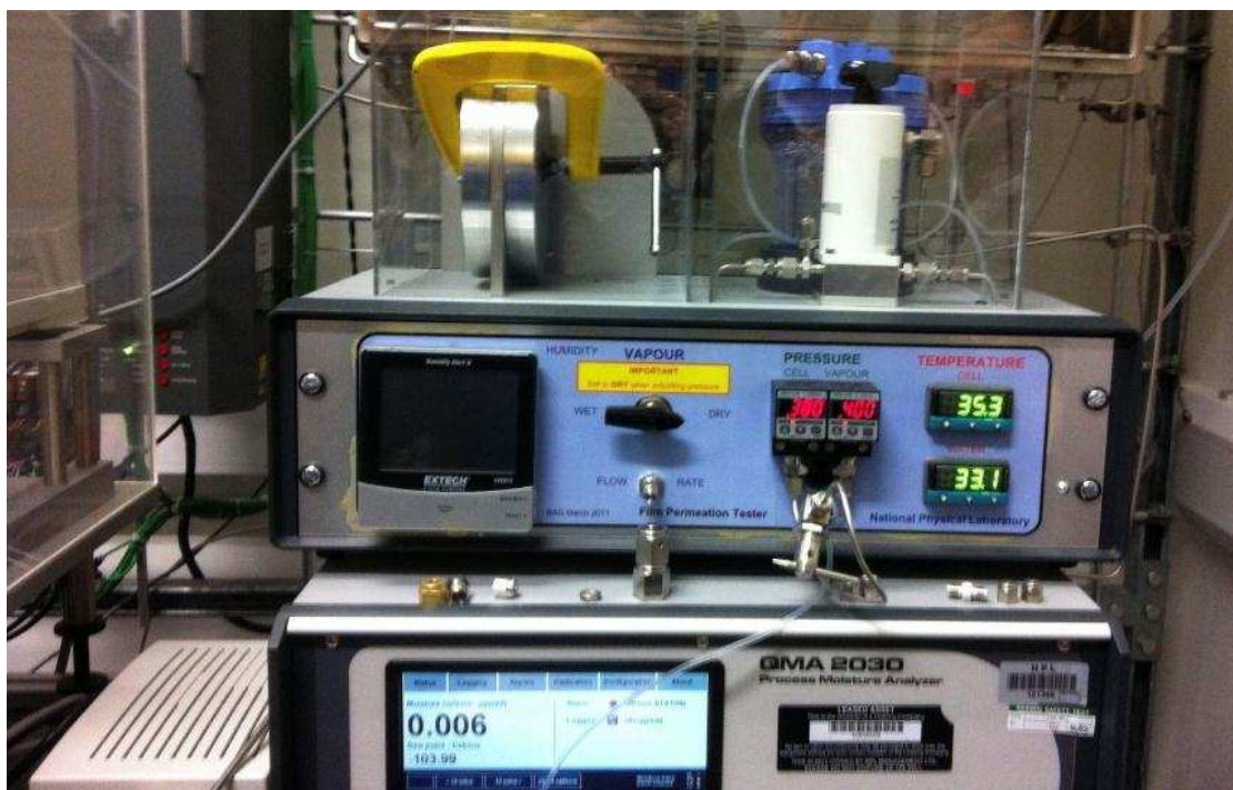
Figure 8-13: Traceable in house WVTR measurement instrument
