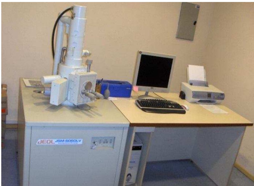
Figure 4-10: The scanning electron microscope—JEOL JSM-6060
