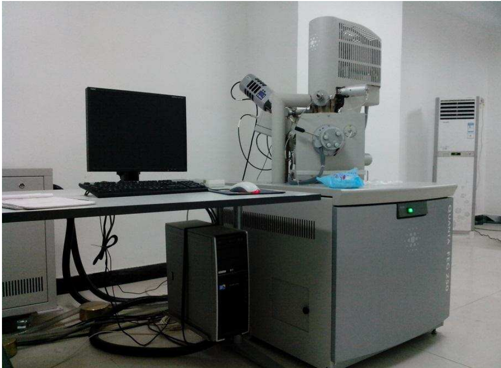
Figure 4-11: The scanning electron microscope — Quanta 250 FEG
