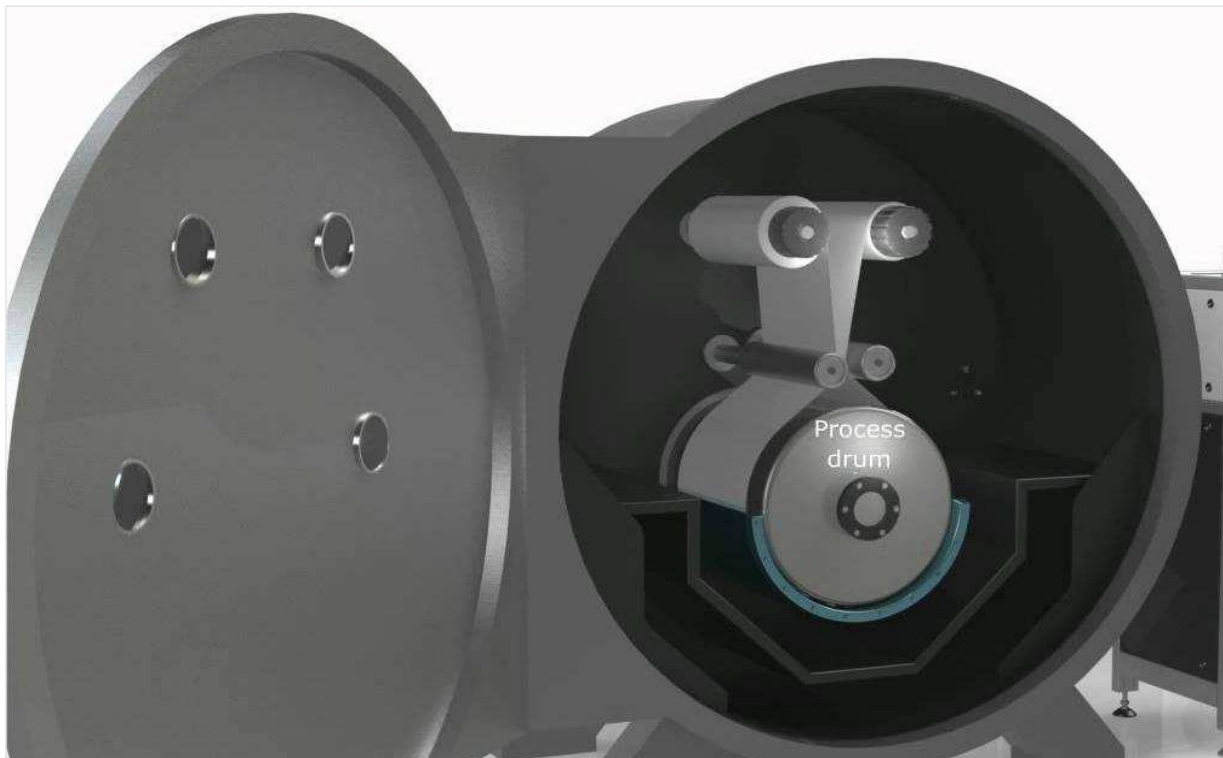
Figure 3-8: Worlds first industrial scale R2R ALD machine WCS 500 (Soininen, 2013)
