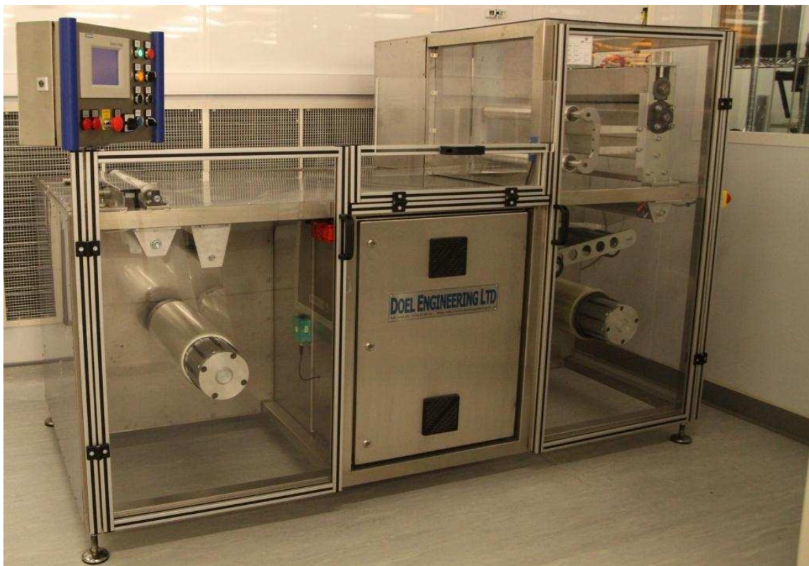
Figure 8-16: Photo of DOEL demonstrator / re-winder
