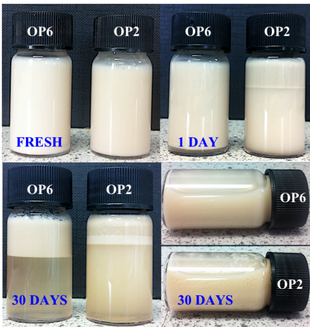
Figure 4.3.3. Macroscopic examination of n -hexadecane-in-water emulsions stored at 25°C.
