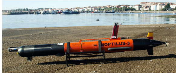
Fig. 1. The human-portable LSTS Light Autonomous Underwater Vehicle (LAUV) [7] is a multi-use vehicle for benthic and upper water-column exploration.
