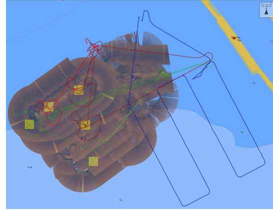
(a) Vehicle trajectory in the second phase of the experiment, overlaid on top of side-scan data (brown) and identified contacts (yellow).
