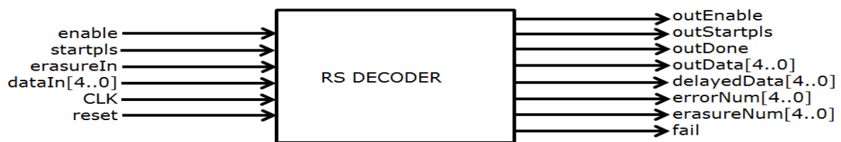
Figure 6.25 RS(31,23) decoder top block view
