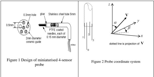
have a protecting PTFE covering there is no requirement for a varnish covering which can roughen the needle surface. To position precisely the four needles utilized as a part of the test, a bored clay aide was utilized as demonstrated as shown in figure 1. The measurements of the
