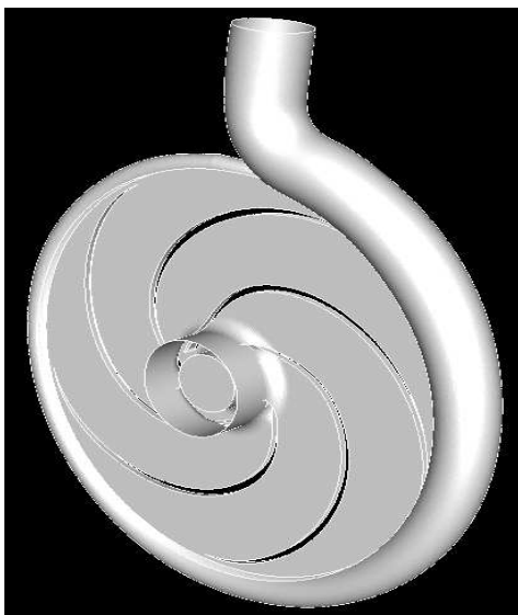
Fig. 1 Numerical model of the pump
