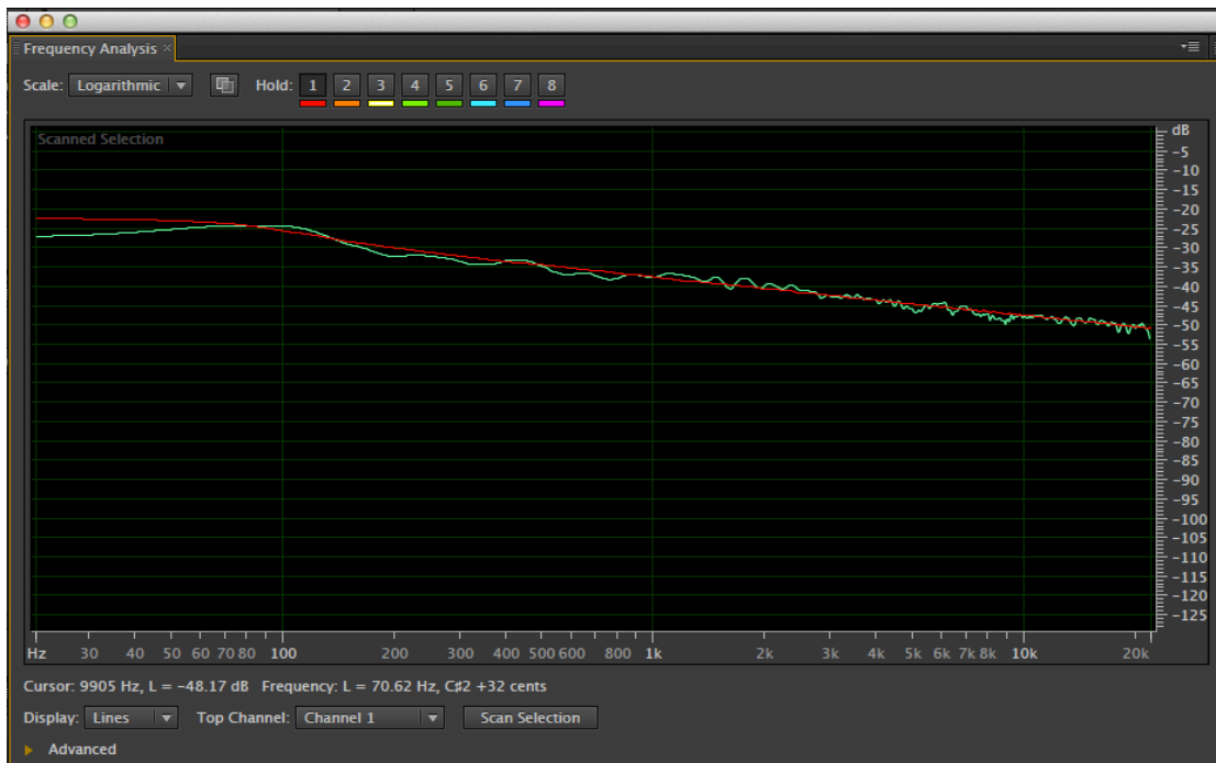
Figure B.3 Second EQ corrections. Note the 300 Hz attenuation has been changed.
