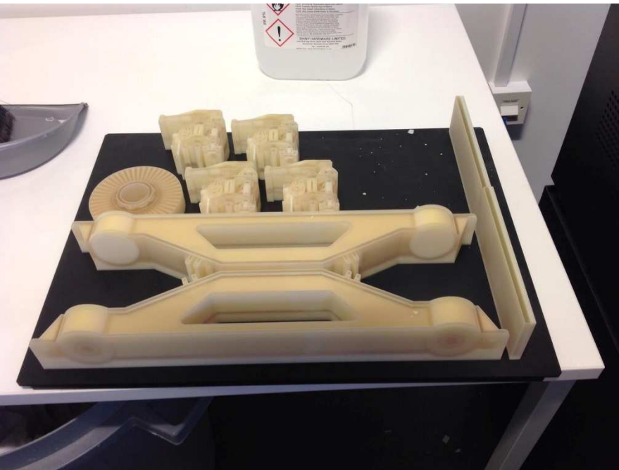
3D printed bogie parts (chassis bearers, brake calipers, brake disc) printed on Projet 5500X Multi Material Printer, at Queen Street Studios, School of Art, Design & Architecture. The train bogie prototype was commissioned by the Institute of Railway, (Dr. Phil Shackleton, Senior Research Fellow, IRR) at University of Huddersfield and funded under the EU FP7 Project Spectrum.
