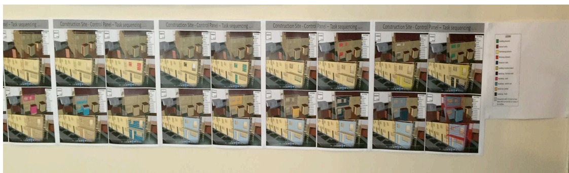
Figure 4: Retrofit work plan produced from screenshots of a 4D model
