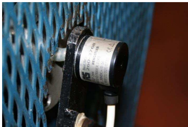
Figure 3.9 Hengstler encoder sensor
