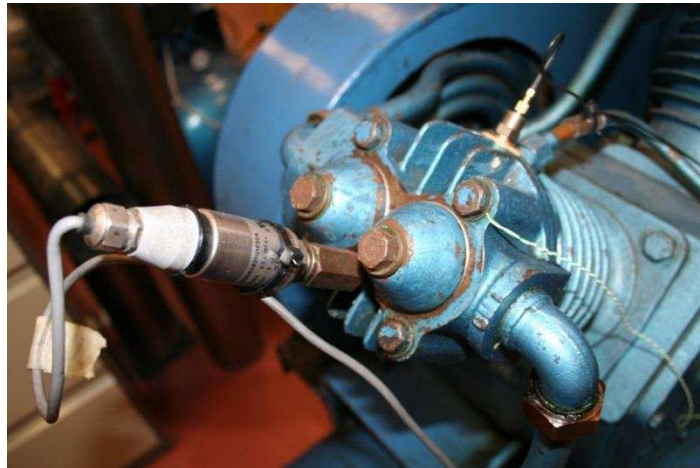
Figure 3.6 Dynamic pressure sensor on cylinder head
