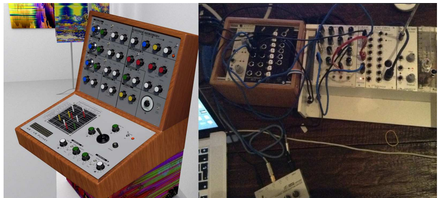
Fig. 4 Virtual analogue VCS3 (left) and Hordijk's Benjolin controlled via an Expert Sleepers digital-to-analogue module.
