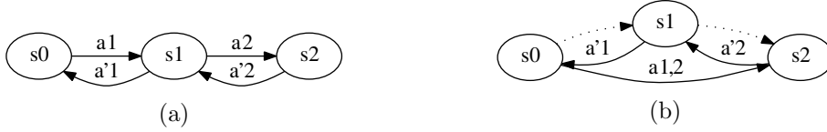
Fig. 1. Replacing primitive actions a_1 and a_2 (a) by a macro-action a_{1,2} (b). Removed primitive actions are visualized by a dotted line in (b).
