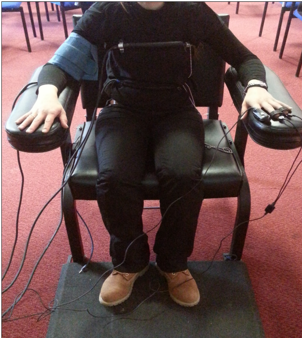
Figure 1: Polygraph Equipment attached to an examinee
