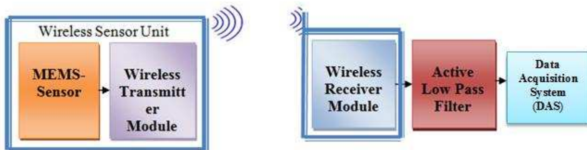
Figure 3.2 Wireless sensing system block diagram.
