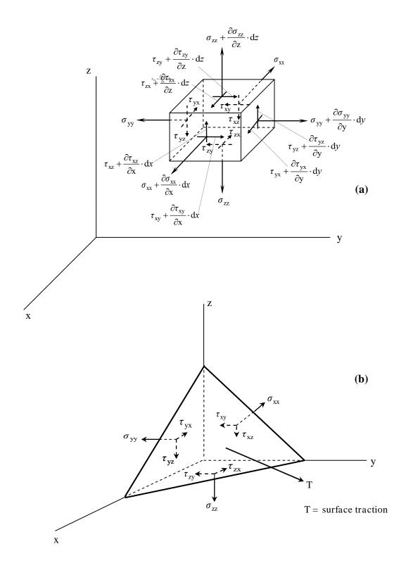
Fig. 1: (a) The total stresses on the boundary surface of an infinitesimal element.
