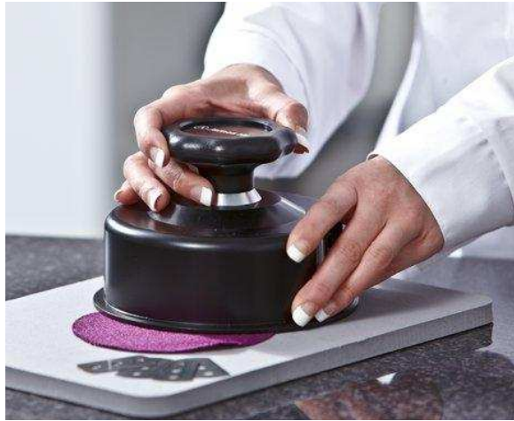
Figure 6: Fabric cutter for creating samples for determining fabric weight [85]
