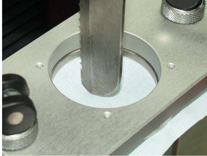
Figure 15: The breadknife just after initial puncture; this was not always the maximum force.
