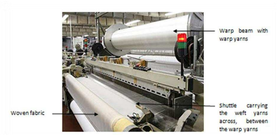
Figure 1: A weaving loom demonstrating the warp and weft directions [95].
