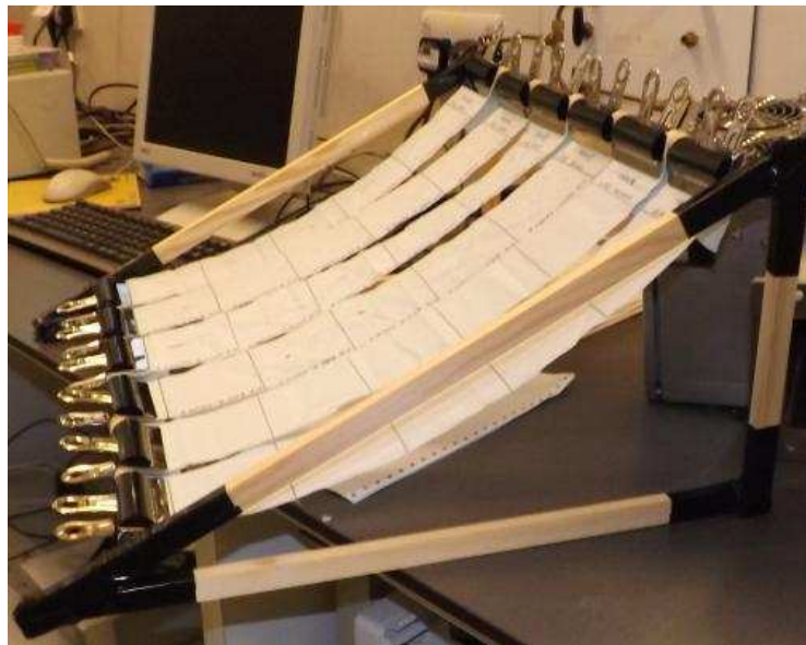
Figure 5: One completed frame before outdoor exposure displaying the 26^{\circ} angle of elevation.
