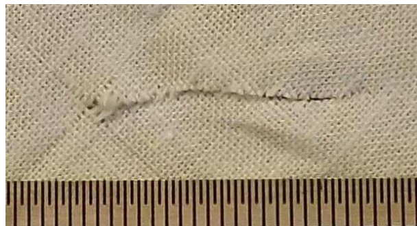
Figure 72: Before outdoor exposure: a wavy stab cut in the bias direction, created with a single edged blade. Each complete division = 1mm.
