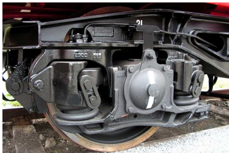
Figure 44: A suspension with double Lenoir links
