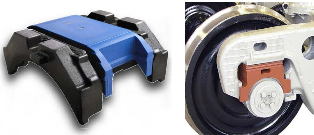
Figure 33: Adapter Plus ® by Amsted (left) and layered shear pad in Russian 18-9800 bogie (right).
