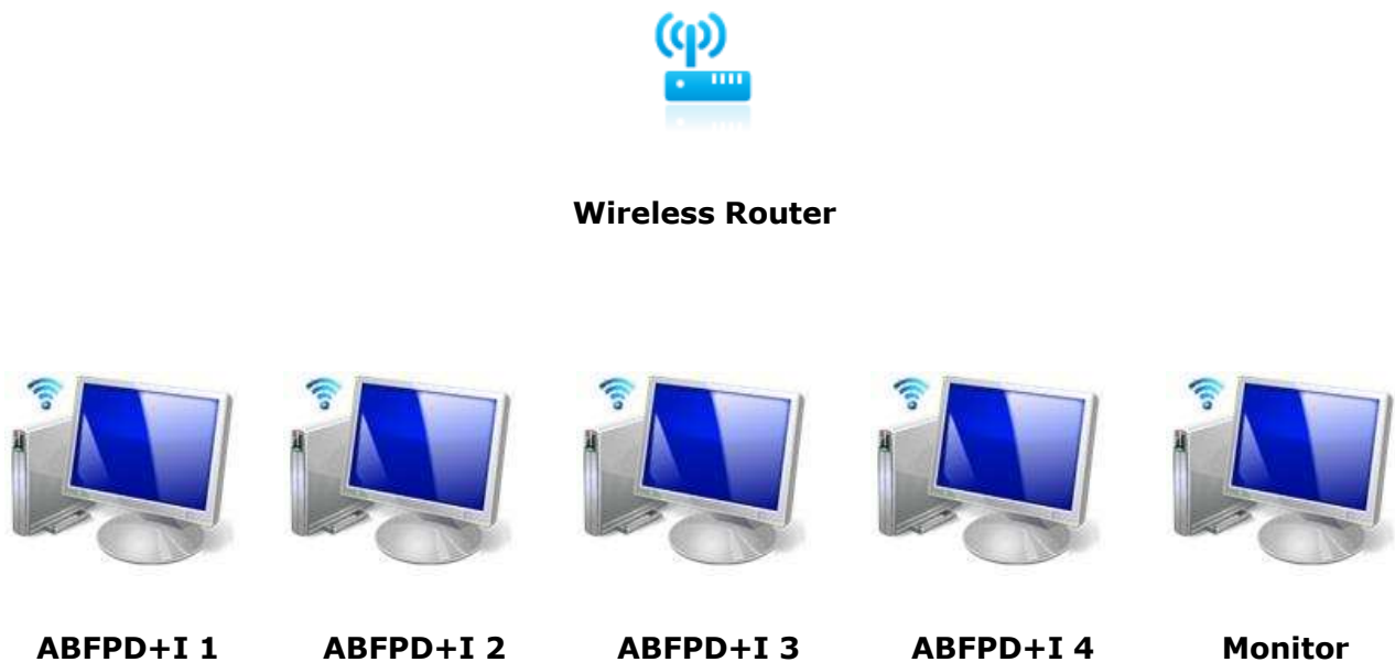
Figure 5-11: The wireless fuzzy logic controller network structure.
