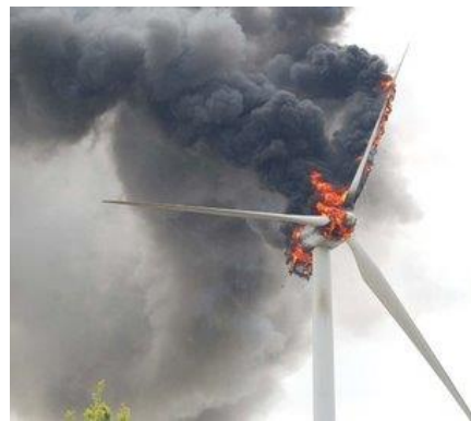
Figure 1.19: Wind Turbine Fire [1.18]
