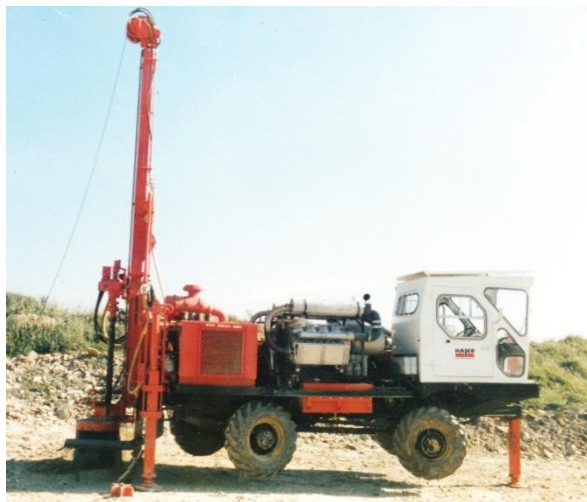
Figure 4.10: Water Well Rock Drill [4.5]
