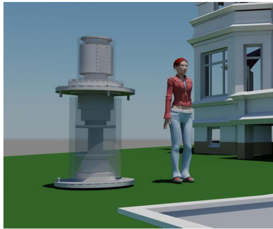
Figure 1.22: Idealised Flywheel Battery 20KWh Storage [1.19]
