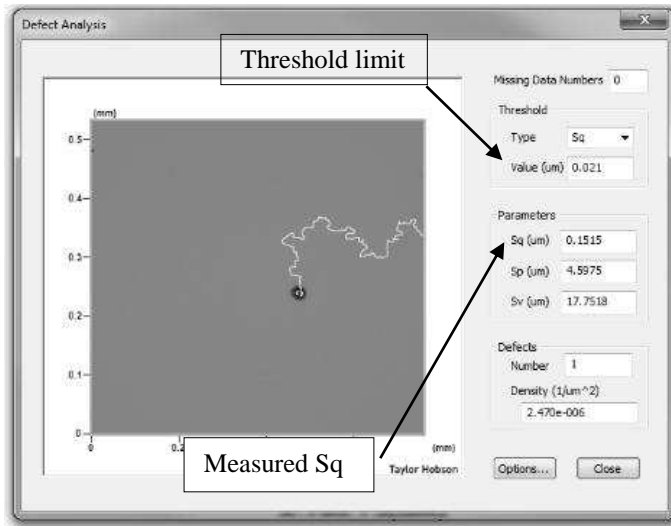
Figure 5: Defect extraction using data segmentation (edge processing and wolf pruning)
