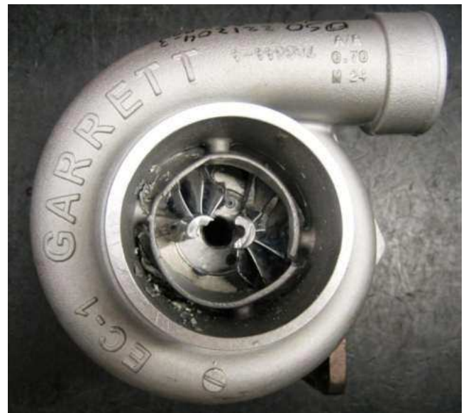
Figure 4 Compressor impeller failure (taken from [5])
