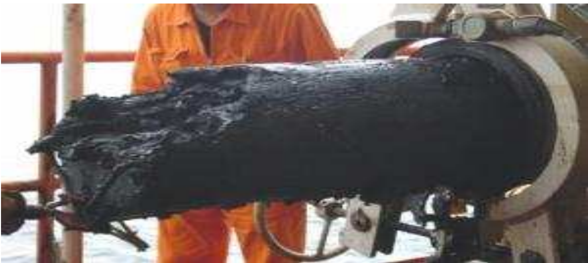
Figure 1.5 Pipe blocked due to the paraffin and asphaltene buildup inside the walls of the pipes[27]
