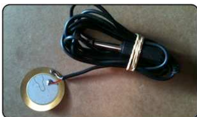
Figure 15 | Piezo-electric microphone used in the harp |
