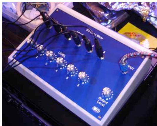
Figure 16 | My custom-made, purpose-built piezo mic mixer |
