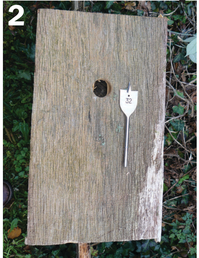
1 Use mortar to make the wall cavity the right size and shape. 2 A piece of old floorboard cut to size makes a good – and free – cover for the nestbox. A 32 mm diameter drill bit was used to make the hole. You can use different sizes to attract various bird species. The British Trust for Ornithology advises the following hole sizes: 25 mm or larger for Blue, Coal and Marsh Tits; 28 mm or larger for Great Tit and Tree Sparrow; and 32 mm for House Sparrow (see www.bto.org/about-birds/nbw/make-a-nest-box ). 3 Left-over mortar can be used to seal the sides and top, while the bottom remains open to provide ventilation. Remember that you'll need to remove the cover once the birds have left to clean out the old nest.
