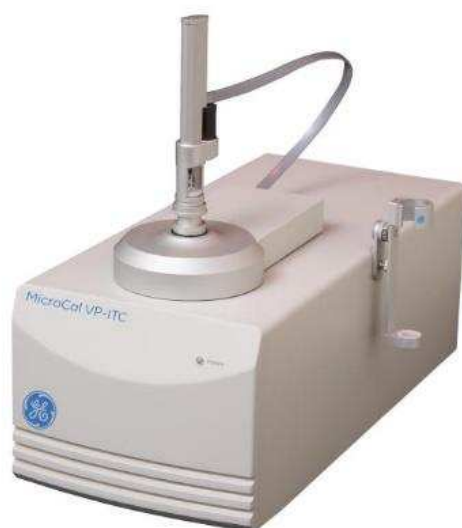
Figure 2.5: A MicroCal VP-ITC used in this study to investigate the thermodynamics of drug-excipient interactions.
