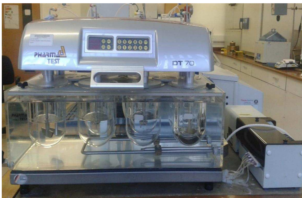
Figure 2.4: Dissolution apparatus used for analysing formulations.
