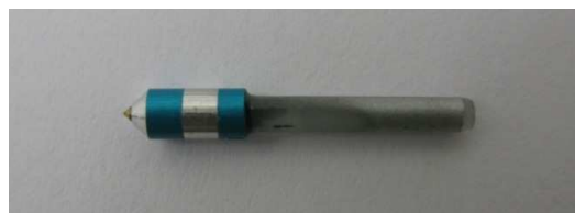
Figure 2.8 The probe, showing a conventional diamond stylus and Zerodur rod
