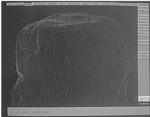
Figure 14: Point Data from Photogrammetric study of Stonehenge. Surveying Stonehenge by Photogrammetry
