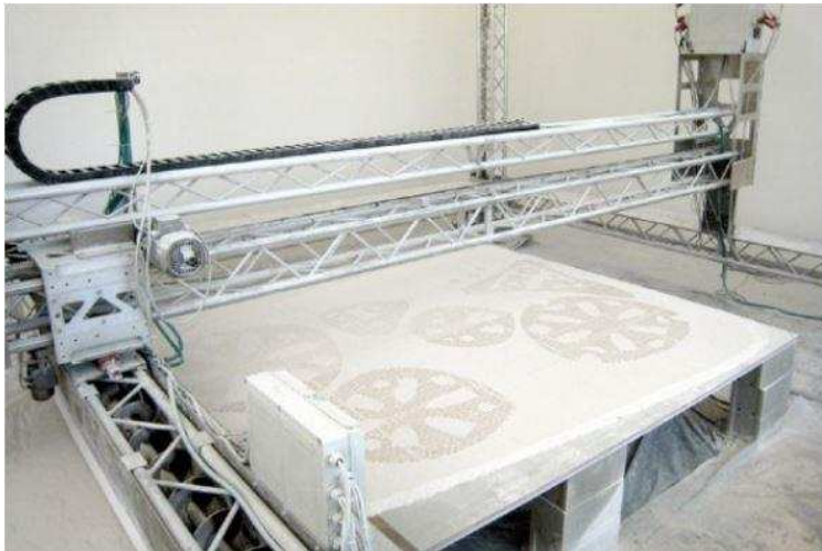
Figure 31: RP Manufacturing: Sand bound together to create a marble-like material
