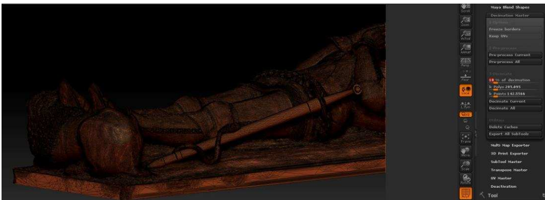
Figure 79: The level of decimation to the right at 10%. Polymesh display shows mesh triangulation.
