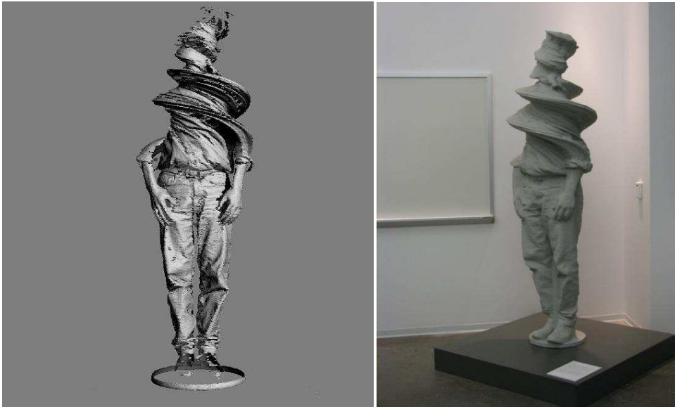
Figure 30: Dan Collins Twister. Original scan data and Finished CNC foam with polyurethane coating
