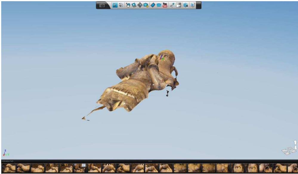
Figure 63: Initial results showing some success with point registering with Automatic Tie Point Extraction in 123D Catch
