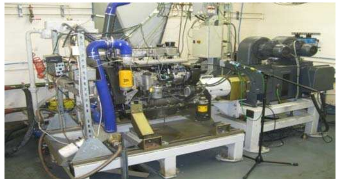
Figure 7. Photo of test rig, Schenk dynamometer fitted with JCB 444 TCA 74kW engine
