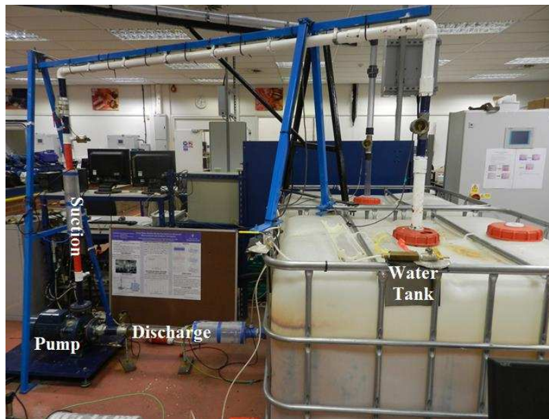
Figure 2 Photo of the pump test rig
