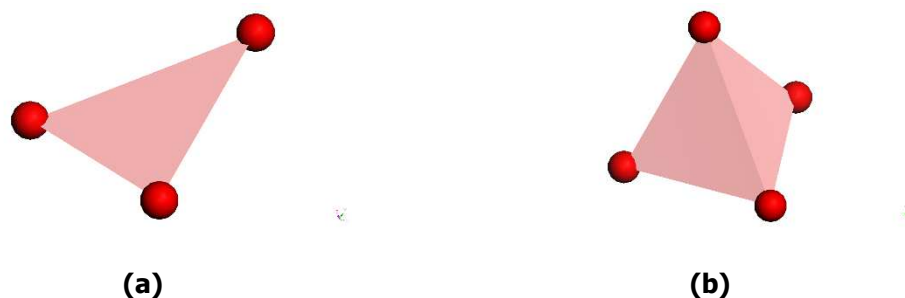
Figure 1.8: Visual representations of: (a) three-coordinated boron and (b) four-coordinated boron.
