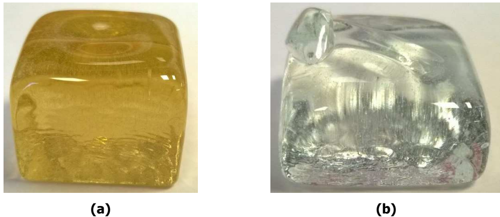
Figure 4.1: Photographs of: (a) MW- \frac{1}{2} Li and (b) Ca/Zn- \frac{1}{2} Li glass ingots. Note the yellow tint in the MW- \frac{1}{2} Li glass ingot due to iron impurities.
