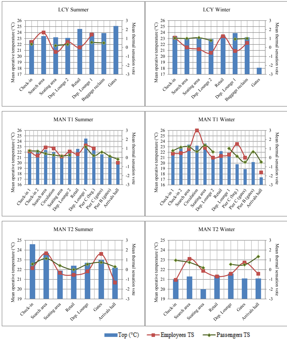
Fig. 2. Mean thermal sensation (lines) for passengers and staff plotted against mean operative temperature (bars) in the monitored terminal spaces. Line breaks indicate insignificant number of questionnaires from the respective population group in the corresponding space.
