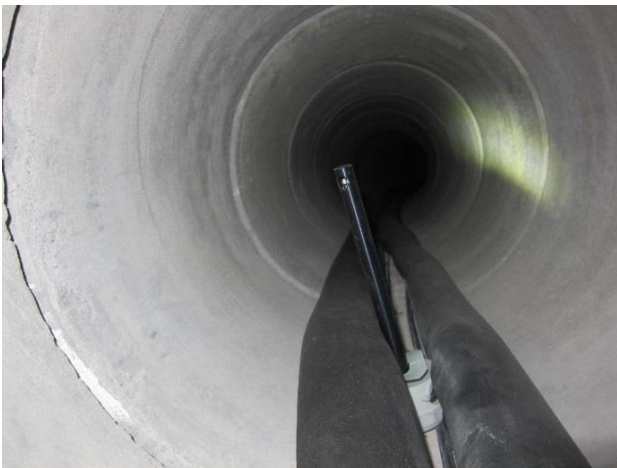
Fig 6: The 'permanent' or fixed anemometer in the tube
