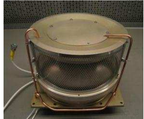
The Electron Analyser System for the Solar Wind Analyser on Solar Orbiter, currently being built at MSSL. Image credit: MSSL.
