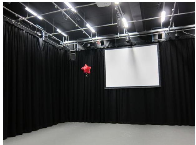
Fig 5: Air movement testing in the dance studio using neutrally buoyant balloons.
