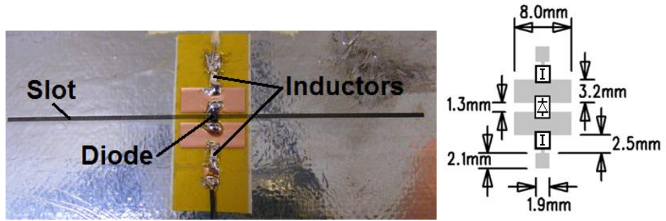
Fig. 3.12. Structure of overlay showing capacitive pads, PIN diode, inductive chokes and bias wires [32].
