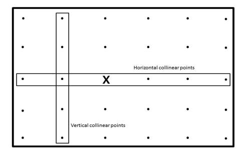
Figure 5.1 Vertical and Horizontal Collinear set of points
